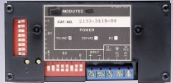
2100 Series with DIP switch selections and multiple power options.
