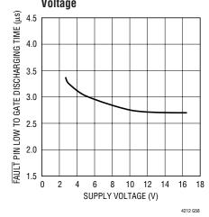
**FAULT** Pin Low to GATE
