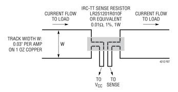
Figure 7. Making PCB Connections to the Sense Resistor
