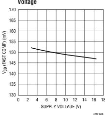
SLOW COMP Trips to GATE Discharging Delay vs Supply Voltage
