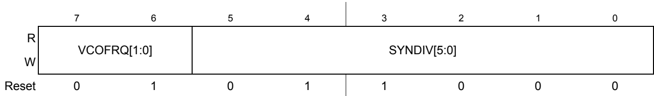
Figure 7-5. S12CPMU_UHV_V5 Synthesizer Register (CPMUSYNR)
