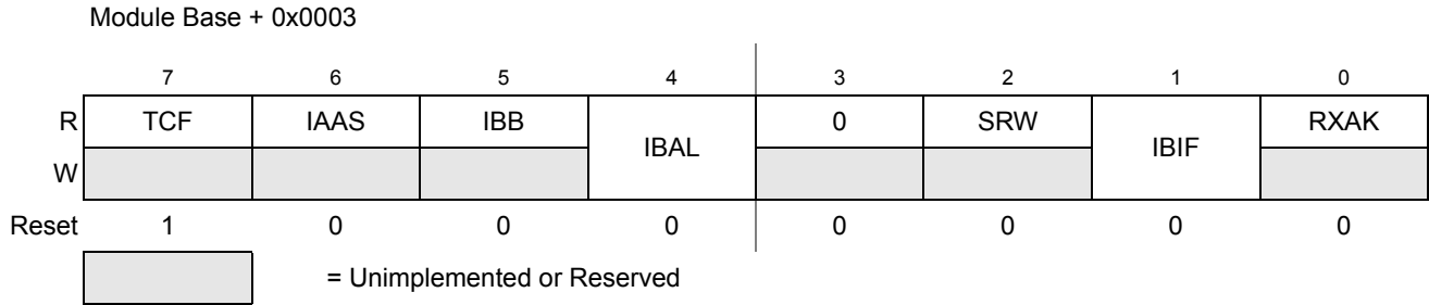
Figure 14-7. IIC Bus Status Register (IBSR)
