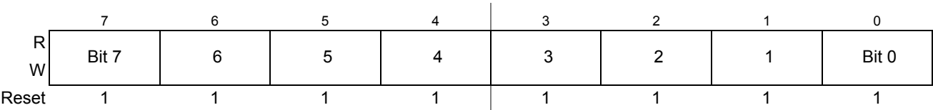
Figure 9-13. PWM Channel Period Registers (PWMPERx)
