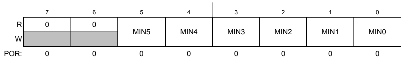
Figure 18-11. Minute Register (MINR)
