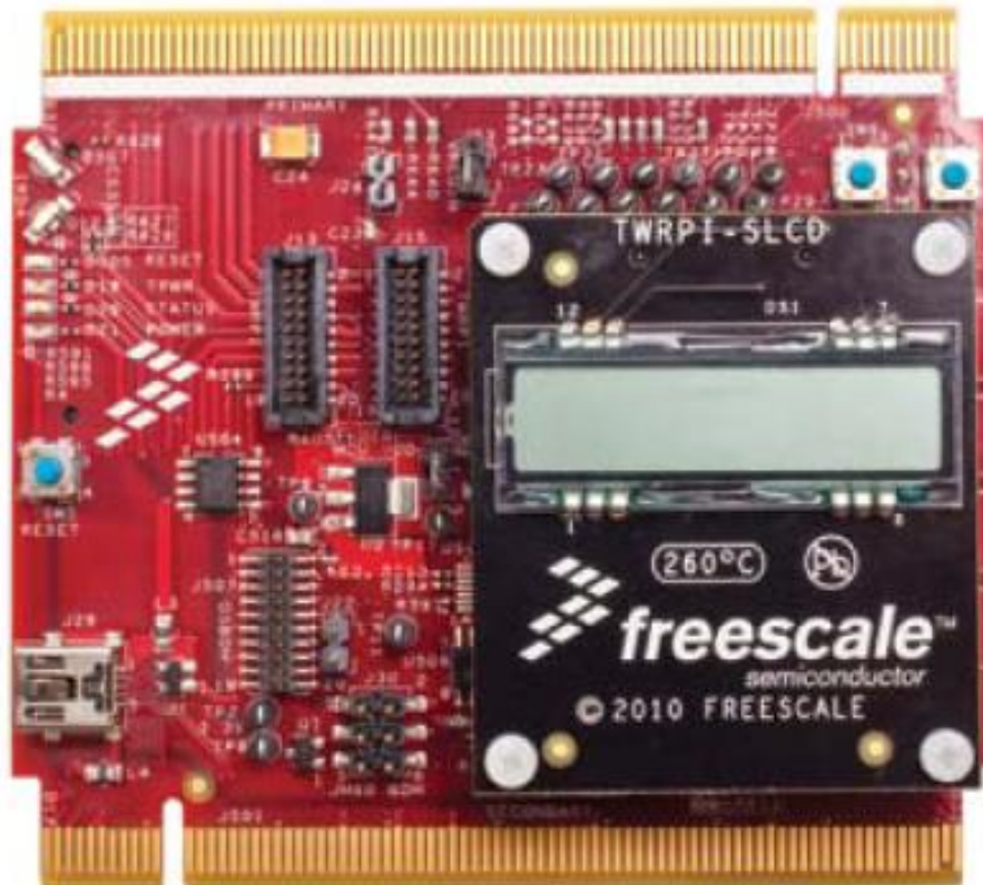
Figure 2: Front side of TWR-K40X256 Module with TWRPI-SLCD attached.
