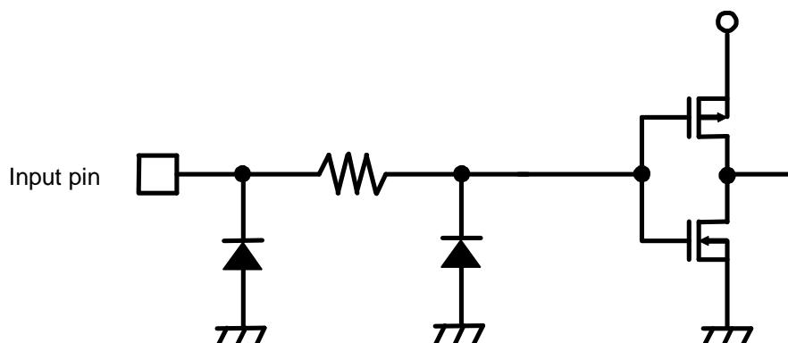
The S-75L04ANC is an inverter fabricated by utilizing advanced silicon-gate CMOS technology which provides the inherent benefit of CMOS low power consumption to achieve operation by only a couple of batteries (1 to 3 V).
