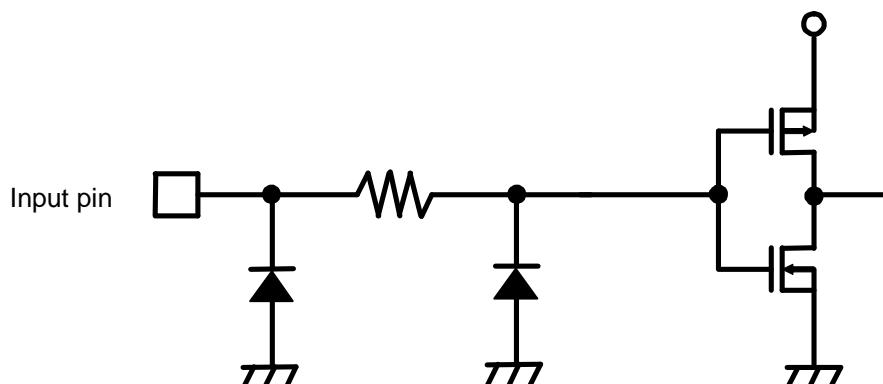
The S-75VU04ANC is a inverter fabricated by utilizing advanced silicon-gate CMOS technology which provides the inherent benefit of CMOS low power consumption to achieve ultra high speed operation correspond to LSTTL IC's.
