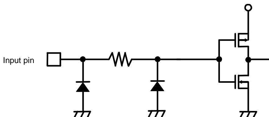
The S-75L14ANC is a SCHMITT INVERTER fabricated by utilizing advanced silicon-gate CMOS technology which provides the inherent benefit of CMOS low power consumption to achieve operation by only a couple of batteries (1 to 3 V).
