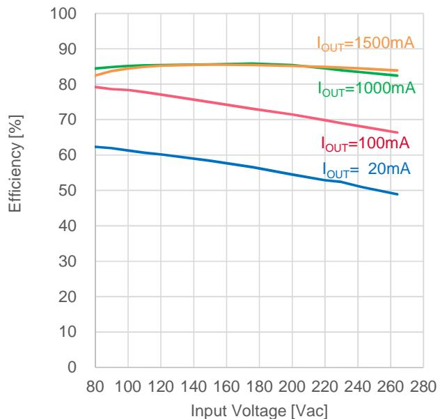
Figure 13. LINE Regulation ( $I_{OUT}$  vs. Efficiency)
