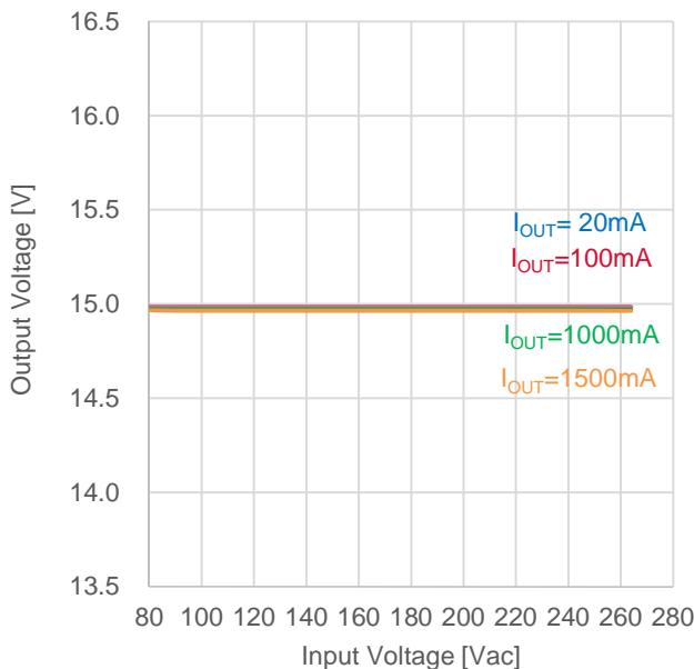
Figure 12. LINE Regulation ( $I_{OUT}$  vs.  $V_{OUT}$ )
