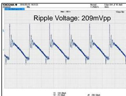
Figure 23. VOUT Ripple Voltage.6
