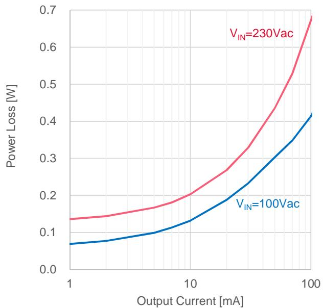
Figure 11. LOAD Regulation ( $I_{OUT}$  vs.  $P_{LOSS}$ )
