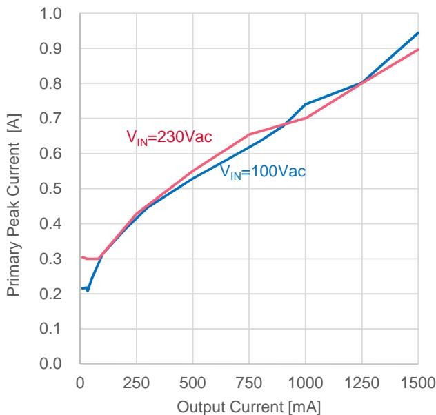
Figure 15. Primary Peak Current ( $I_{OUT}$  vs.  $I_{peak}$ )
