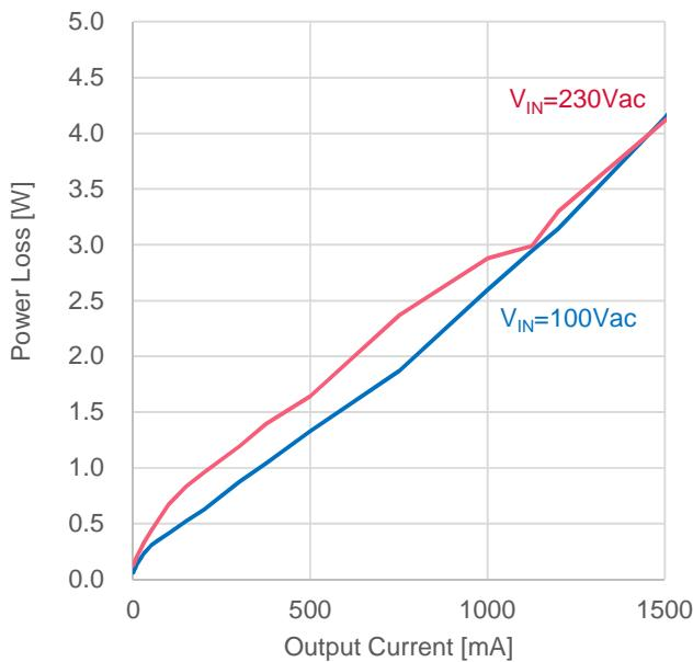
Figure 10. Load Regulation ( $I_{OUT}$  vs.  $P_{LOSS}$ )
