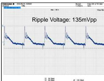
Figure 22. VOUT Ripple Voltage.5
