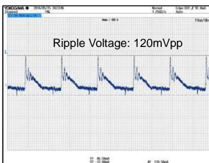
Figure 19. VOUT Ripple Voltage.2
