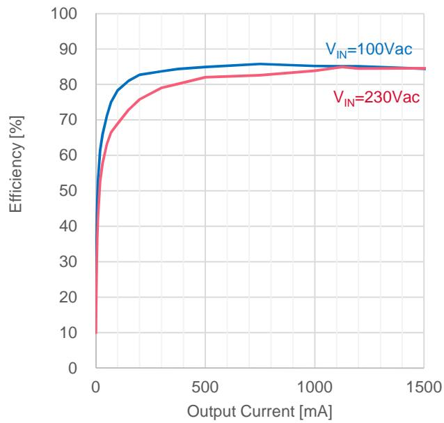
Figure 9. LOAD Regulation ( $I_{OUT}$  vs. Efficiency)Table 3. Load Regulation ( $V_{IN}=100\text{Vac}$ )
