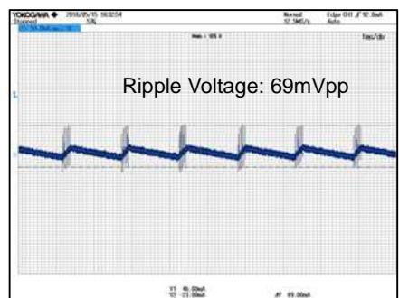
Figure 21. VOUT Ripple Voltage.4
