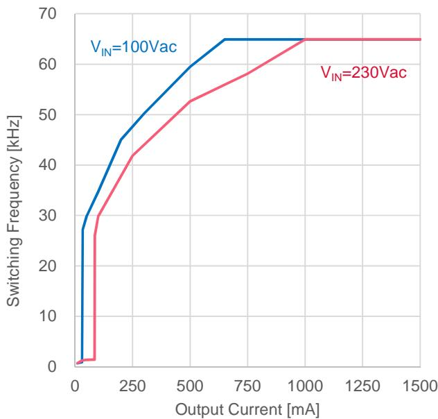
Figure 14. Switching Frequency ( $I_{OUT}$  vs.  $F_{SW}$ )
