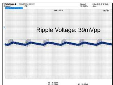
Figure 18. VOUT Ripple Voltage.1
