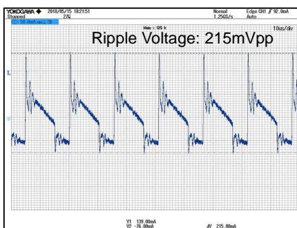
Figure 20. VOUT Ripple Voltage.3
