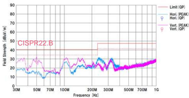
Figure 26. Radiated Emission.1
