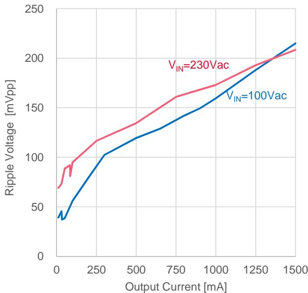
Figure 17. VOUT Ripple Voltage ( $I_{OUT}$  vs.  $V_{ripple}$ )
