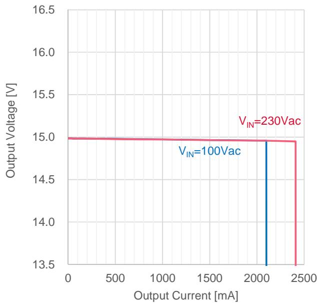
Figure 8. Load Regulation ( $I_{OUT}$  vs.  $V_{OUT}$ )
