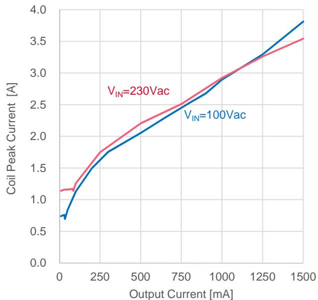
Figure 16. Secondary Peak Current ( $I_{OUT}$  vs.  $I_{peak}$ )
