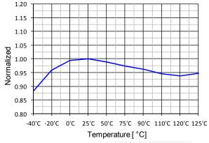
Figure 8. Peak Drain Current Limit (ILIM) vs. TA
