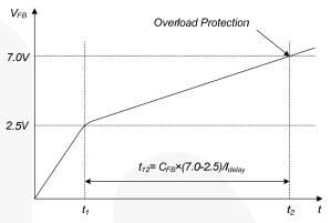
Figure 20. Overload Protection
