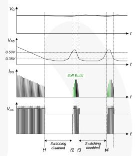
Figure 23. Burst Mode Operation
