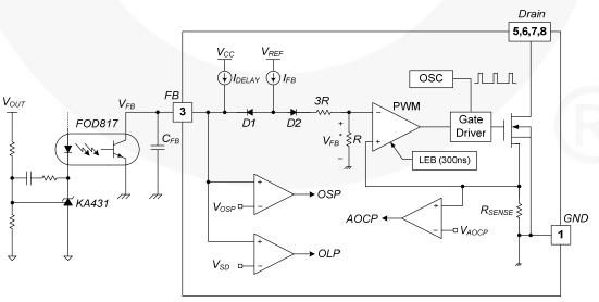
Figure 18. Pulse Width Modulation Circuit
