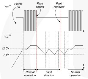
Figure 19. Auto-Restart Protection Waveforms
