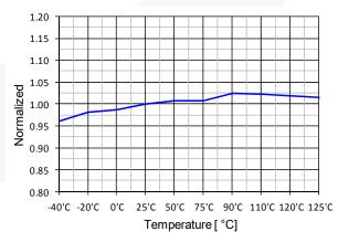
Figure 10. Shutdown Delay Current (IDELAY) vs. TA
