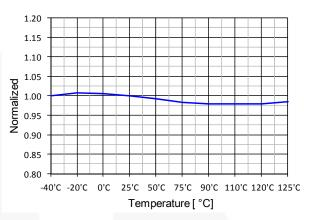
Figure 6. Operating Switching Current ( $I_{OPS}$ ) vs.  $T_A$
