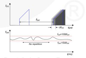
Figure 24. Random Frequency Fluctuation
