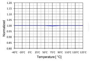
Figure 15. Switching Frequency (fs) vs. TA
