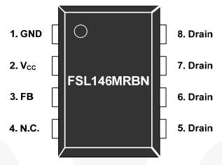
Figure 3. Pin Configuration (Top View)
