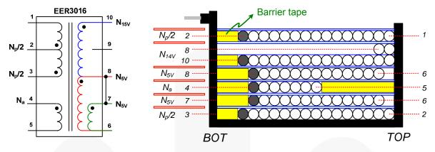
Figure 26. Schematic of Transformer
