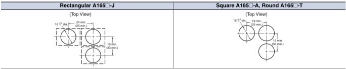
Note: 1. Make sure the thickness of the mounting panel is 0.5 to 3.2 mm.
