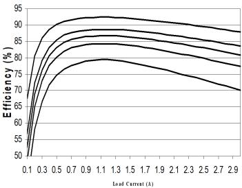
Efficiency versus Load, VIN = 3.3V
