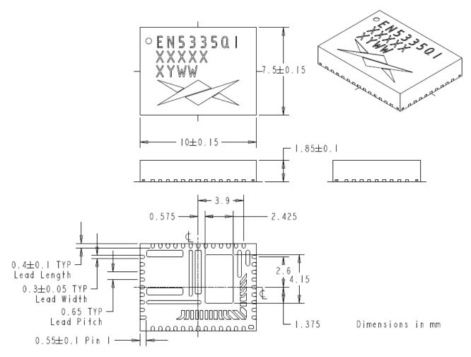
Figure 7: EN5335QI Package Dimensions (Bottom View)
