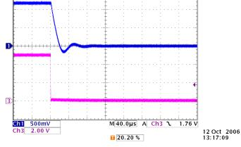
Start-up waveform, V<sub>IN</sub>/V<sub>OUT</sub> = 5.5V/1.2V
