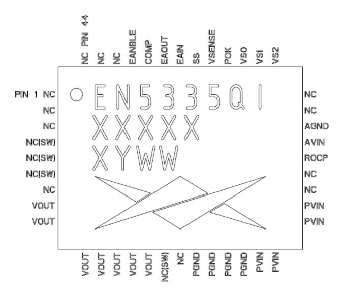
Figure 2: Pin Diagram (Top View)
