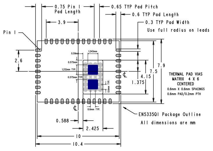
Figure 6: EN5335QI PCB Footprint (Top View)
