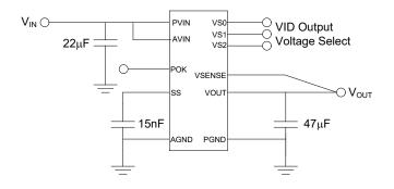
**Figure 1: Simplified Applications Circuit**
