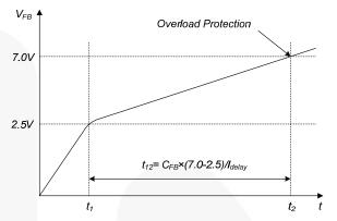
Figure 22. Overload Protection
