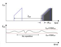
Figure 27. Random Frequency Fluctuation
