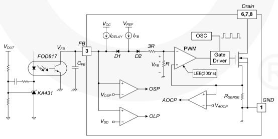
Figure 20. Pulse Width Modulation Circuit
