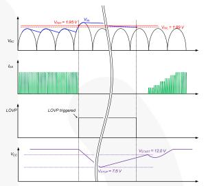
Figure 25. Line Over-Voltage Protection
