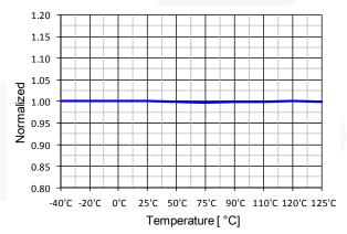
Figure 16. Maximum Duty Ratio (D<sub>MAX</sub>) vs. T<sub>A</sub>
