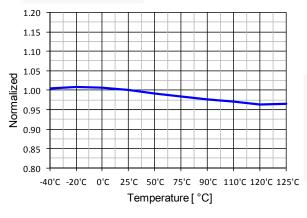
Figure 15. Switching Frequency (fs) vs. TA
