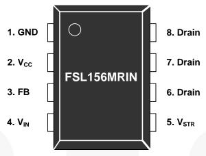
Figure 3. Pin Assignments (Top View)
