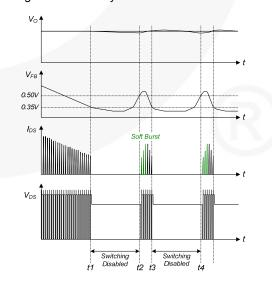
Figure 26. Burst-Mode Operation
