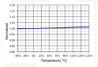
Figure 12. UVLO Threshold Voltage (V<sub>STOP</sub>) vs. T<sub>A</sub>
