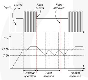
Figure 21. Auto-Restart Protection Waveforms
