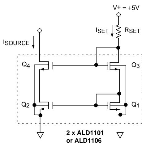
Q<sub>1</sub>, Q<sub>2</sub>, Q<sub>3</sub>, Q<sub>4</sub>: N - Channel MOSFET
