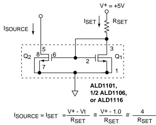
Q<sub>1</sub>, Q<sub>2</sub> : N - Channel MOSFET
