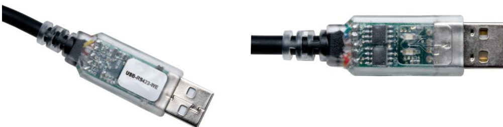
Figure 5.3 USB-RS422-WE Cable images
