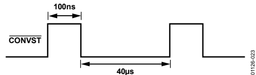
Figure 21. \overline{\text{CONVST}} When Temperature Channel Selected
