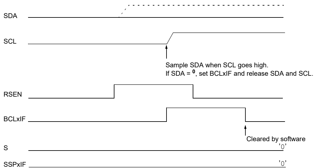
Figure 35-36. Bus Collision During a Repeated Start Condition (Case 1)
