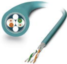
Bus system cable, ETHERNET, 4-pos., PUR halogen-free blue, 2x2x26 AWG, cable ring: 100 m
