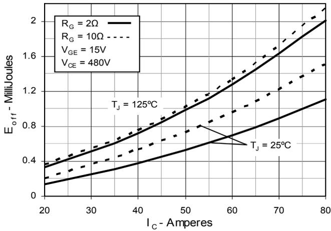
Fig. 10. Dependence of Turn-Off Energy on Temperature
