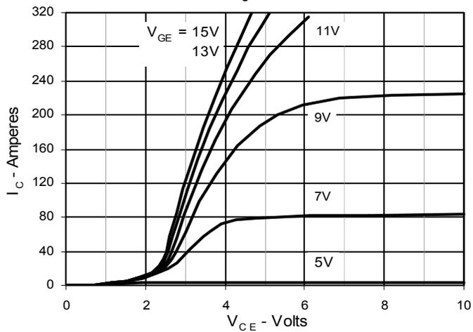
Fig. 3. Output Characteristics
