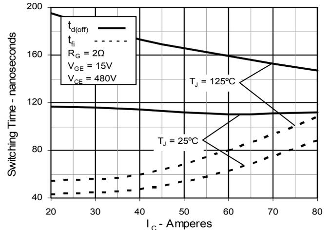
**Fig. 13. Dependence of Turn-Off Switching Time on Temperature**
