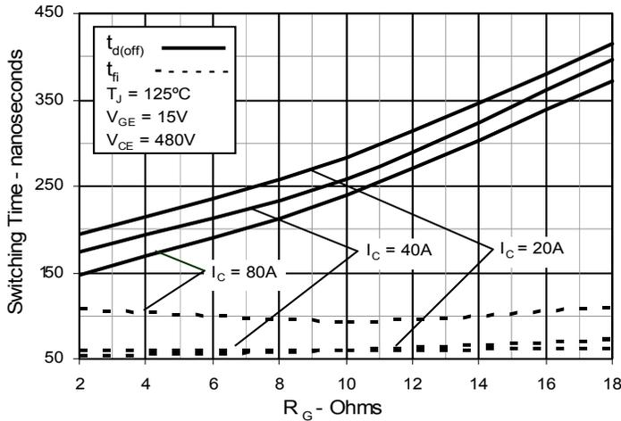
Fig. 12. Dependence of Turn-Off Switching Time on  $I_C$
