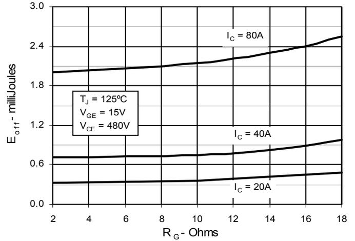
Fig. 9. Dependence of Turn-Off Energy on  $I_C$
