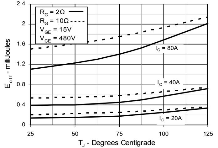
Fig. 11. Dependence of Turn-Off Switching Time on  $R_G$
