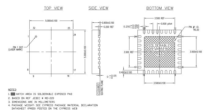
Figure 18. 32-pin QFN ( $5 \times 5 \times 1.0$  mm) Package Outline, 001-30999
