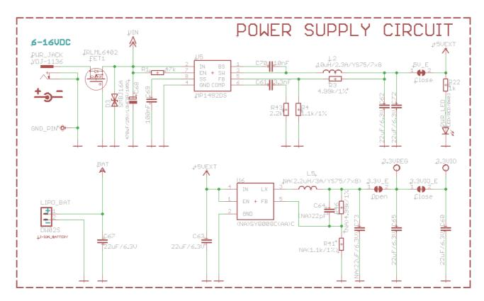
Note that the whole 3.3V part is not mounted (elements marked as NA) by default because we use the internal 3.3V DC-DC convertor in the iMX233. However, the internal DC-DC in the processor
