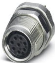
Sensor/actuator flush-type plug-in connector, socket, 8-pos. M8, rear/screw mounting with M10 fastening thread, with straight solder connection
