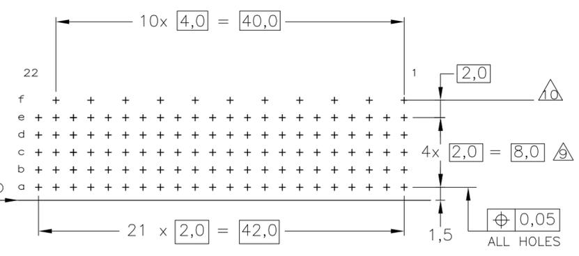
P.C.B. HOLE DIM. ACTION PIN
