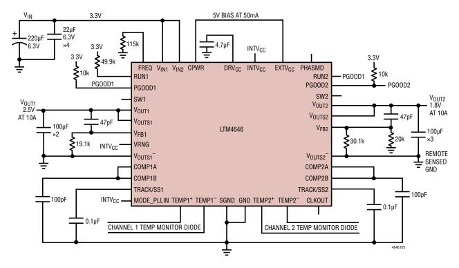
Figure 21. 3.3V to 1.8V, and 2.5V at 10A each with PGOOD Power Up Sequencing
