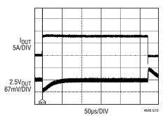
$C_{OUT}$  = 100 $\mu$ F ×2, CERAMIC  $C_{COMP}$  = 100pF,  $C_{FF}$  = 47pF f = 500kHz
