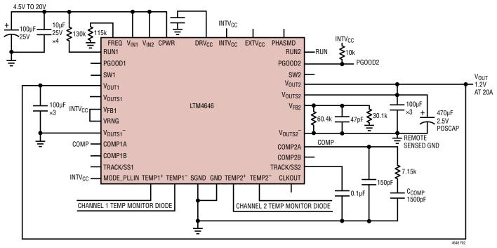
Figure 2. 2-Phase Parallel Configurations
