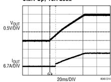
$\begin{array}{l} 12V_{IN}, 1.5V_{OUT} \text{ AT 10A LOAD} \\ C_{OUT} = 470\mu\text{F} \times 1, 2.5\text{V}, \text{SANYO POSCAP}, \\ 100\mu\text{F} \times 4, 6.3\text{V}, \text{CERAMIC} \\ \text{SOFT-START CAPACITOR} = 0.1\mu\text{F} \\ \text{USE RUN PIN TO CONTROL START-UP} \end{array}$
