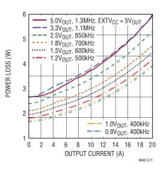
Figure 11. 12V<sub>IN</sub> Power Loss Curve
