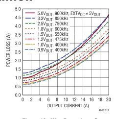
Figure 10.  $8V_{IN}$  Power Loss Curve
