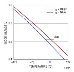
Figure 7. Diode Voltage  $V_D$  vs Temperature T(°C) for Different Bias Currents
