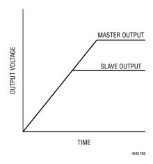
Figure 6. Output Coincident Tracking Waveform
