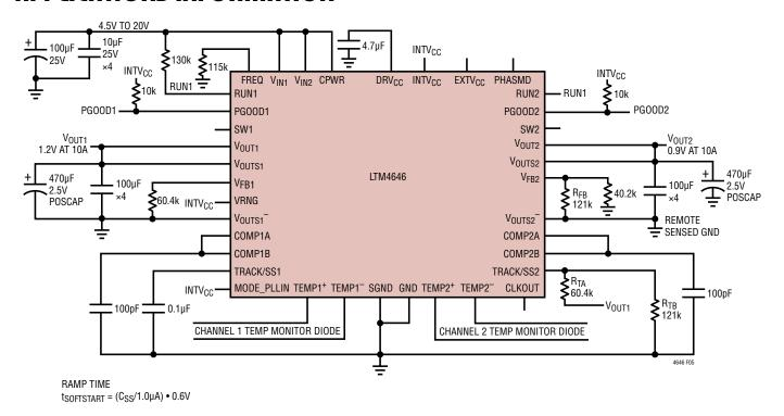
Figure 5. Example of Output Tracking Application Circuit
