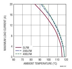
Figure 12. 5V to 1V Derating Curve, No Heat Sink, f<sub>SW</sub> = 350kHz, EXTV<sub>CC</sub> Electrically Connected to V<sub>IN</sub>
