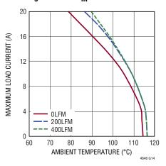
Figure 14. 5V to 2.5V Derating Curve, No Heat Sink, f<sub>SW</sub> = 550kHz, EXTV<sub>CC</sub> Electrically Connected to V<sub>IN</sub>
