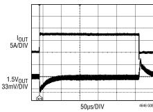
$C_{OUT} = 100 \mu F \times 3$ , CERAMIC  $C_{COMP} = 100pF, C_{FF} = 47pF$ f = 450kHz
