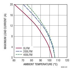
Figure 16. 12V to 5V Derating Curve, No Heat Sink, f<sub>SW</sub> = 1.3MHz, EXTV<sub>CC</sub> Electrically Connected to V<sub>OUT</sub>
