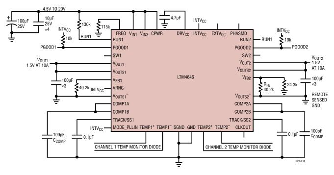
Figure 18. 4.5V to 20V Input to 1.5V Dual Output, at 10A Each
