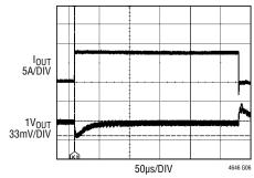
$C_{OUT} = 470 \mu F$  POSCAP,  $5 m\Omega$ , 100μF ×4, CERAMIC C<sub>COMP</sub> = 100pF, f = 350kHz
