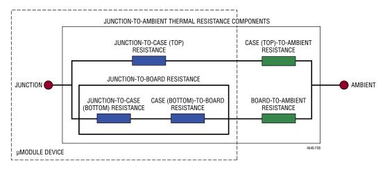
Figure 8. Graphical Representation of JESD51-12 Thermal Coefficients
