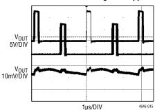
12V TO 1V AT 20A TWO-PHASE 12V TO 1V AT 350kHz RIPPLE AT 20A LOAD  $C_{OUT}=330\mu F, 9m\Omega, 100\mu F \times 4, CERAMIC$
