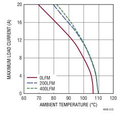
Figure 15. 12V to 2.5V Derating Curve, No Heat Sink, f<sub>SW</sub> = 850kHz
