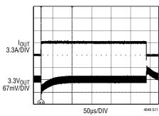
$C_{OUT}$  = 100 $\mu$ F ×1, CERAMIC  $C_{COMP}$  = 100pF,  $C_{FF}$  = 47pF f = 750kHz
