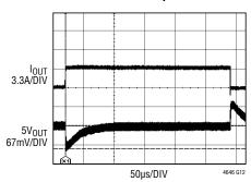
$C_{OUT}$  = 100 $\mu$ F ×1, CERAMIC  $C_{COMP}$  = 100pF,  $C_{FF}$  = 47pF f = 950kHz
