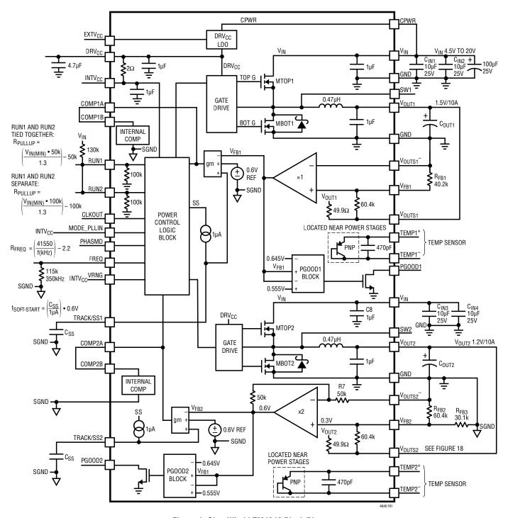
Figure 1. Simplified LTM4646 Block Diagram
