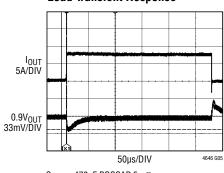
$C_{OUT} = 470 \mu F POSCAP, 5 m\Omega$ 100μF ×4, CERAMIC  $C_{COMP} = 100pF,$ f = 350kHz
