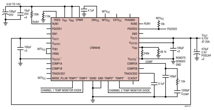
Figure 19. 12V Input to 0.75V at 20A Two Phase
