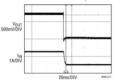
$V_{IN} = 12V$   $V_{OUT} = 1.5V$   $I_{OUT} = 10A$
