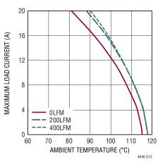
Figure 13. 12V to 1V Derating Curve, No Heat Sink, f<sub>SW</sub> = 400kHz
