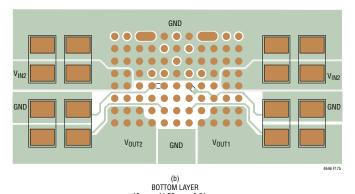
Figure 17. Recommended PCB Layout
