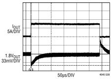
$C_{OUT} = 100 \mu F \times 3$ , CERAMIC  $C_{COMP} = 100pF, C_{FF} = 47pF$ f = 500kHz
