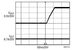
$12V_{\text{IN}},~1.5V_{\text{OUT}}$  at no load  $C_{\text{OUT}}=470\mu\text{F}\times\text{1},~2.5\text{V},~\text{SANYO POSCAP},~100\mu\text{F}\times\text{4},~6.3\text{V},~\text{CERAMIC}$  SOFT-START CAPACITOR = 0.1 $\mu\text{F}$  USE RUN PIN TO CONTROL START-UP
