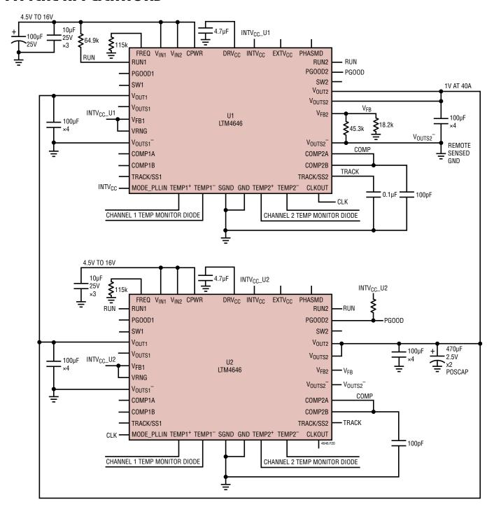
Figure 20. Four Phase Design 1V at 40A
