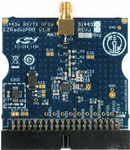
Figure 17. Single-Ended TX and RX Testcard
