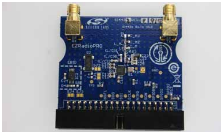
Figure 16. Split TX and RX Testcard (Rx: Left SMA, Tx: Right SMA) for Use with Coaxial Cable and RF Test Equipment for Scientific RF Evaluation (May be Ordered Separately)
