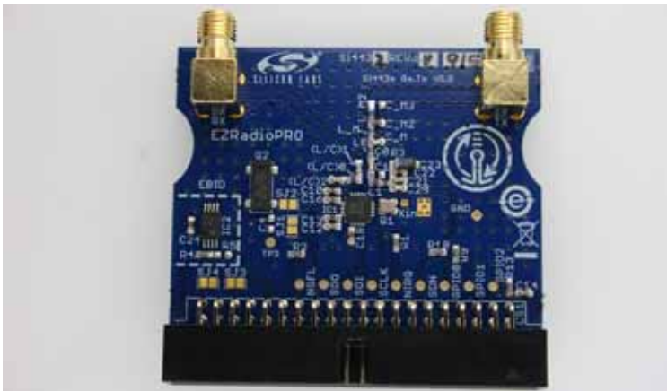
Figure 16. Split TX and RX Testcard (Rx: Left SMA, Tx: Right SMA) for Use with Coaxial Cable and RF Test Equipment for Scientific RF Evaluation (May be Ordered Separately)
