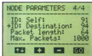
Figure 19. Screen 4: Setting Up the Node Parameters
