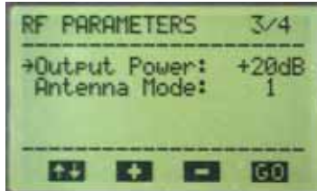
Figure 18. Screen 3: RF Parameters (Antenna Diversity Card Fitted)
