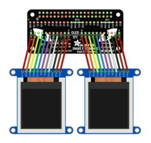
The 1.54" TFT has a 12th pin labeled "TE". DO NOT CONNECT THAT PIN TO THE BONNET. Only connect the other 11 pins from "Vin" through "Lite"
