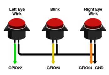
For all buttons, connect one leg of each to **GND**, and the opposite leg to a digital pin:
