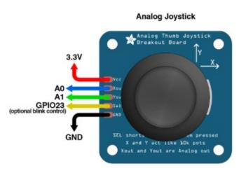
XOUT and YOUT from a joystick can connect to analog pins A0 and A1.
