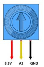
For manual control of pupil dilation (instead of responding to light) a 10K potentiometer can be used. The center leg connects to analog pin **A2** (same input as the photocell, just substituting a different analog control).
