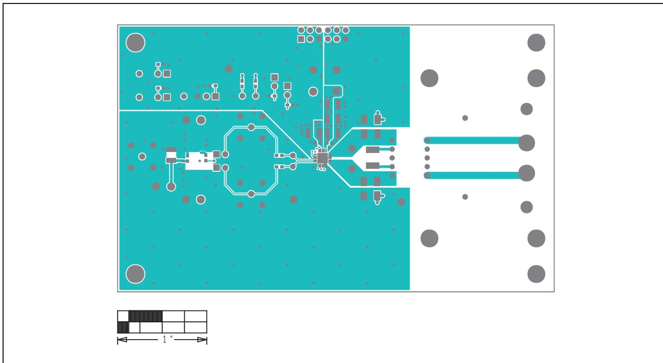
Figure 3. MAX44211 EV Kit PCB Layout—Component Side
