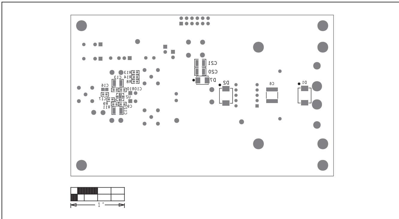
Figure 7. MAX44211 EV Kit Component Placement Guide—Solder Side
