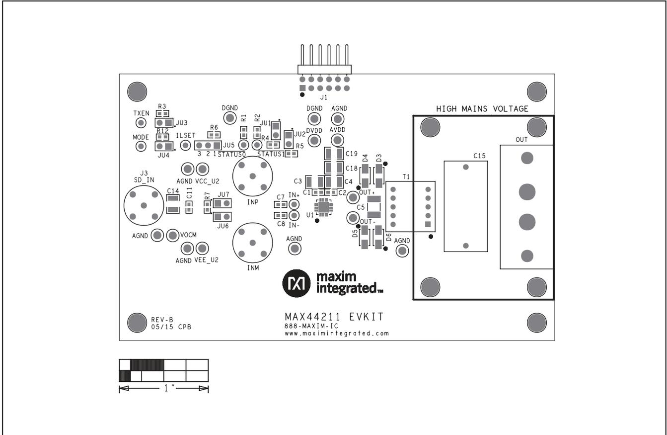
Figure 2. MAX44211 EV Kit Component Placement Guide—Component Side
