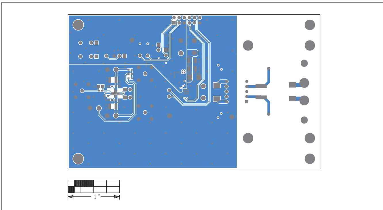
Figure 6. MAX44211 EV Kit PCB Layout—Solder Side
