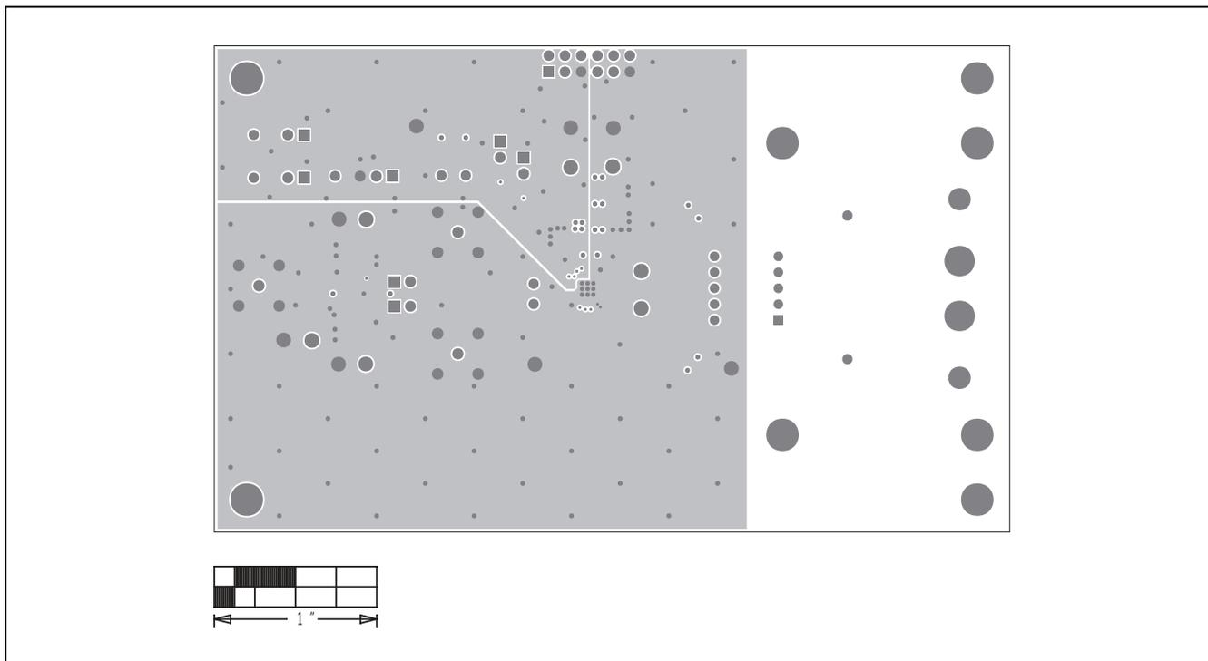
Figure 4. MAX44211 EV Kit PCB Layout—Inner Layer 2
