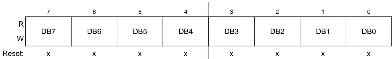
Figure 10-33. Data Segment Registers (DSR0–DSR7) — Extended Identifier Mapping
