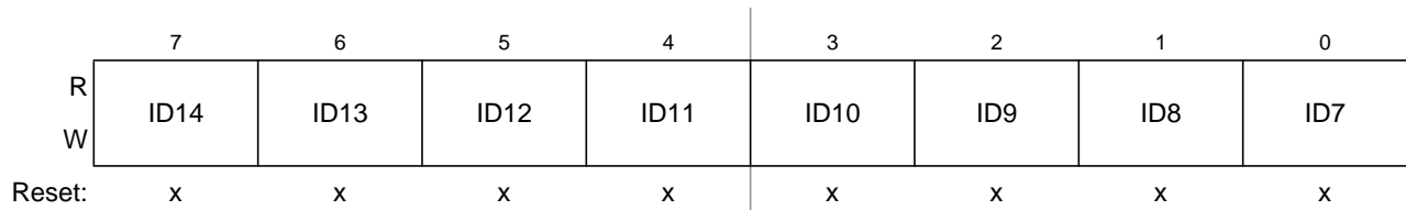
Figure 10-27. Identifier Register 2 (IDR2) — Extended Identifier Mapping
