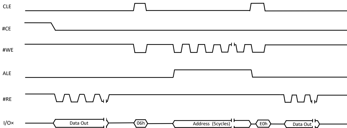
Figure 9-4 Two Plane Random Data Read (06h-E0h) Operation
