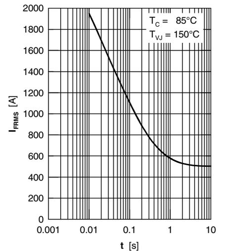
Fig. 5 Rated RMS current versus time (360° conduction)
