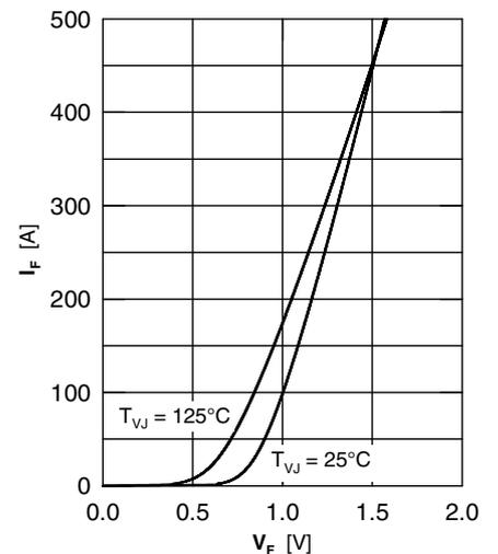
Fig. 7 Forward current versus voltage drop
