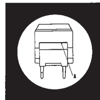
Stand-Off Lugs Minimize Solder-Creepage
