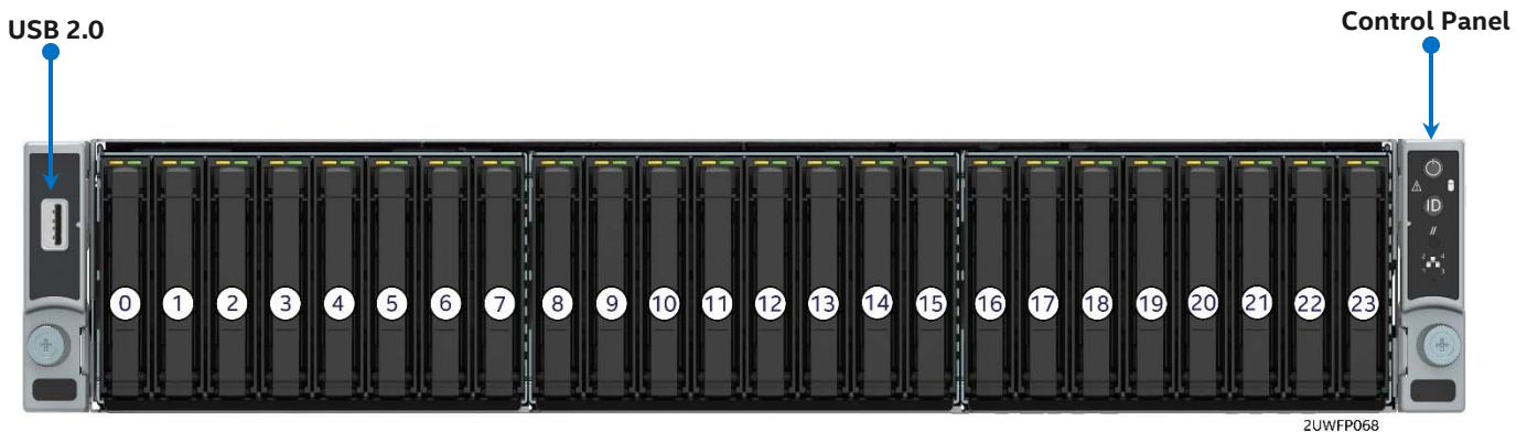
Figure 40. 2.5" front mount drive bay, 24 drive (R2224WFxxx) configuration
