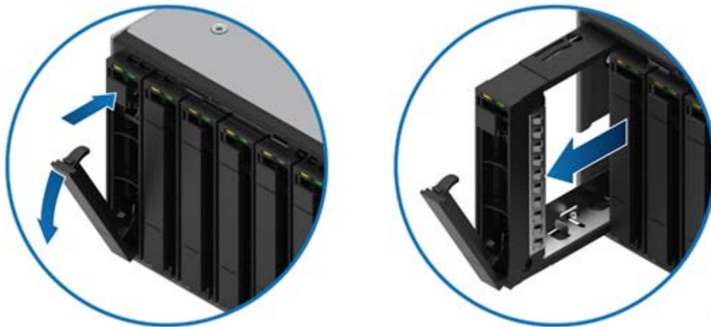
Figure 43. Drive carrier removal
