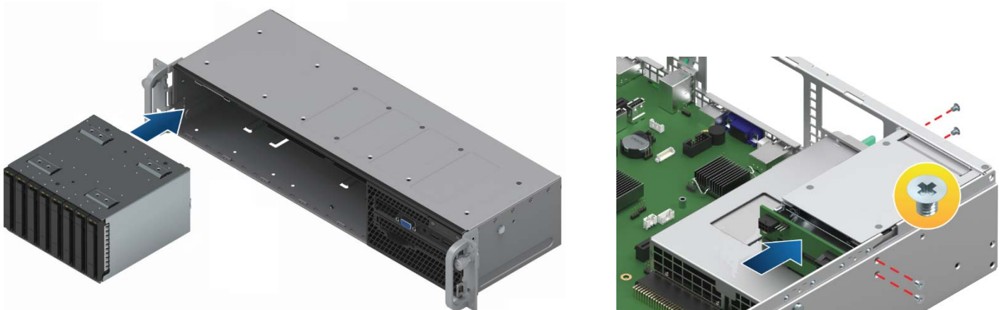
Figure 48. 2.5" drive bay module placement options
