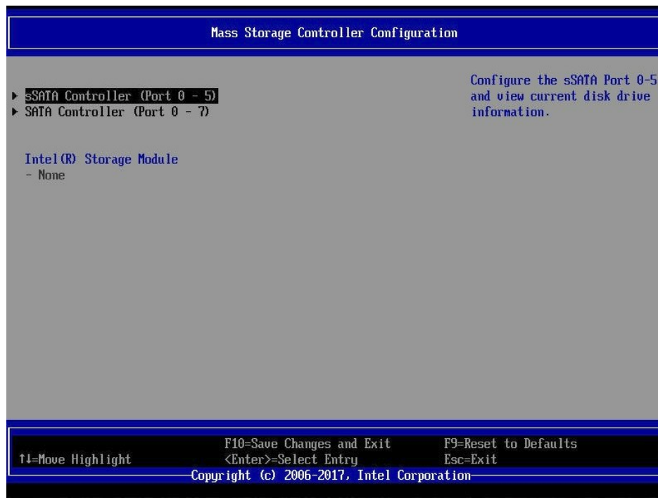
Figure 61. BIOS setup Mass Storage Controller Configuration screen
