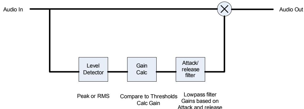
**Figure 9. Compressor block diagram**
