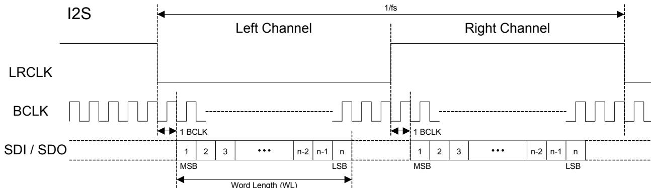
Figure 28. I<sup>2</sup>S Justified Audio Interface (assuming n-bit word length)
