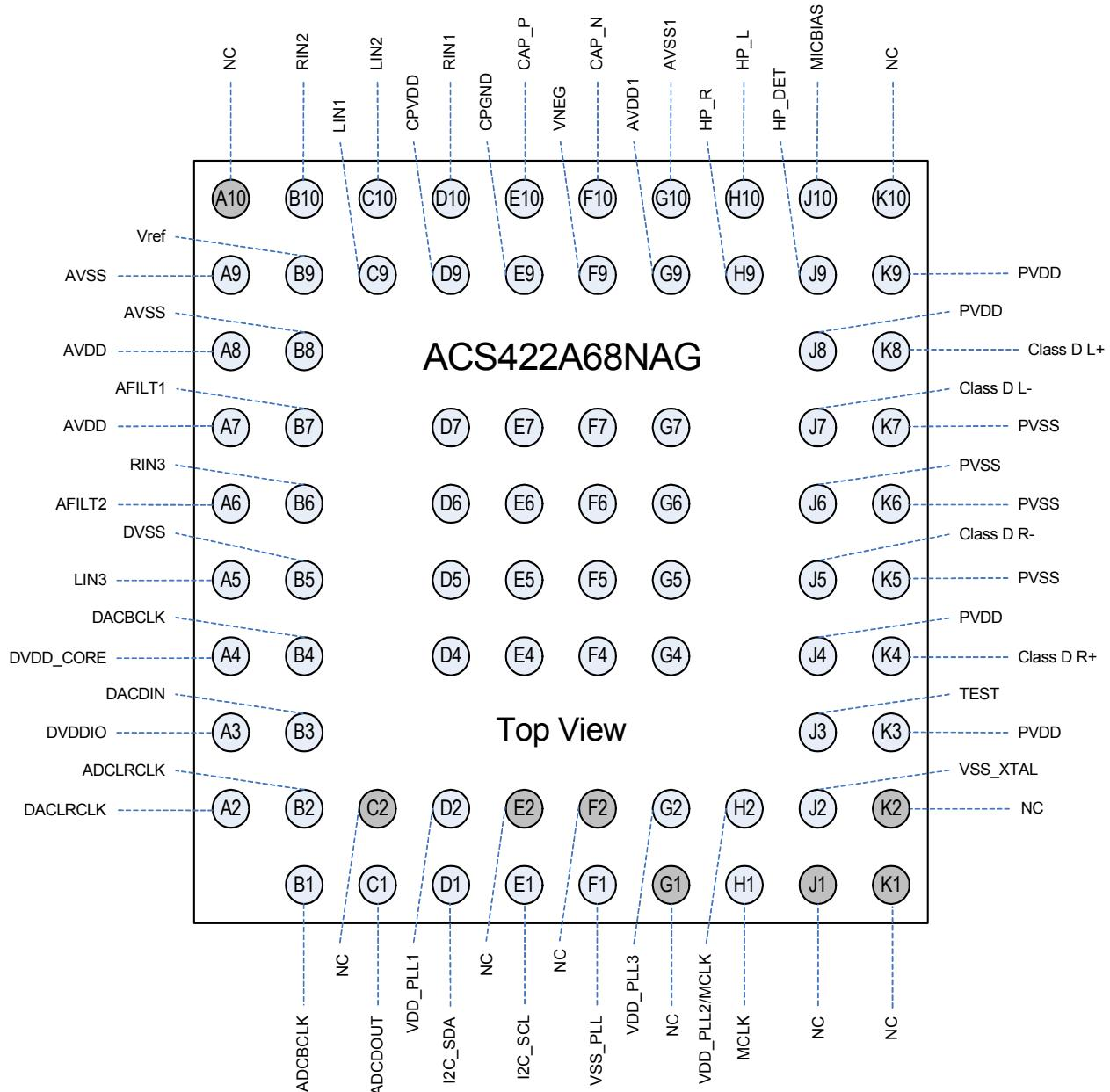
Figure 36. ACS422x68NAG Pinout
