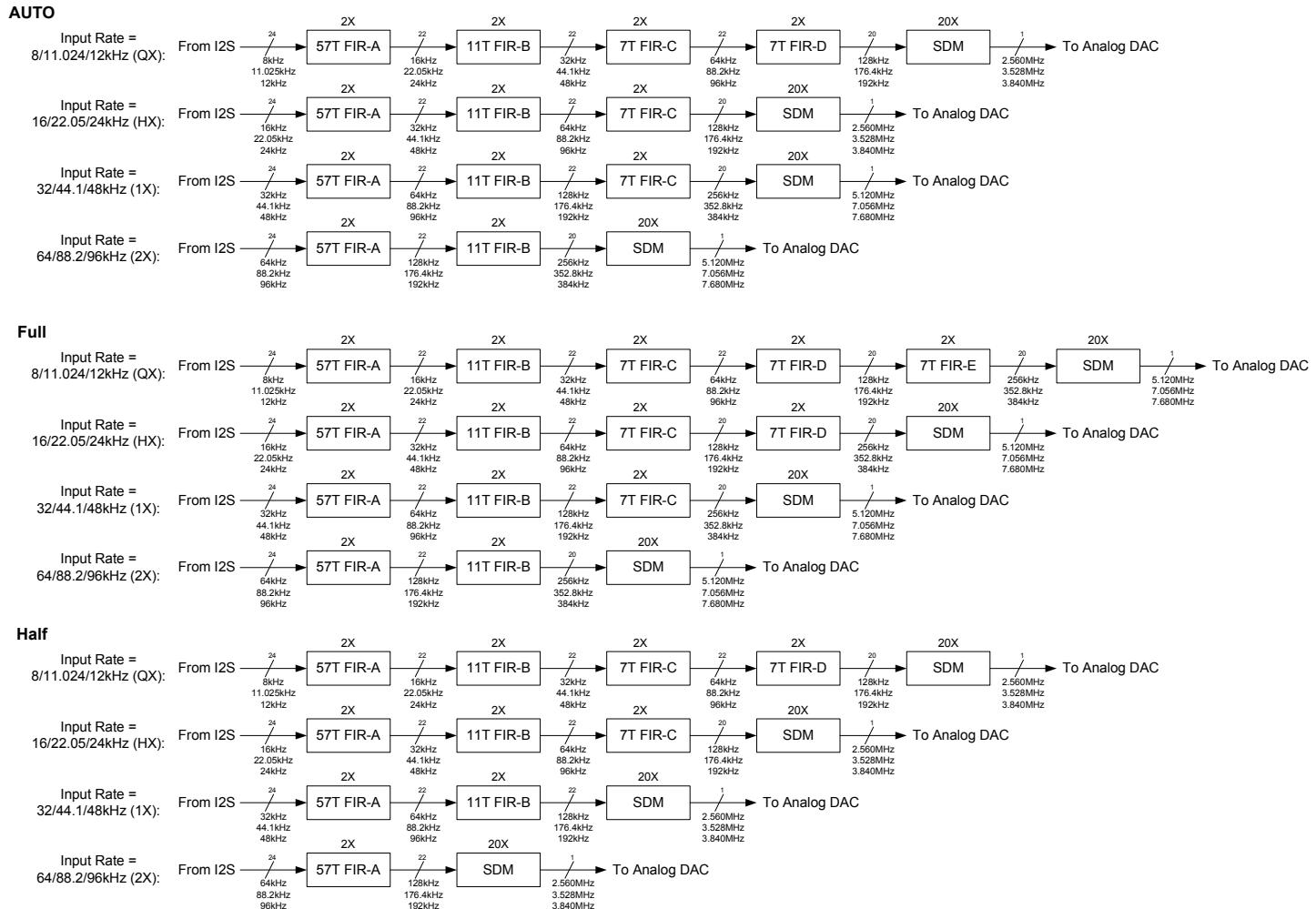
**Figure 13. Interpolation and Filtering**
