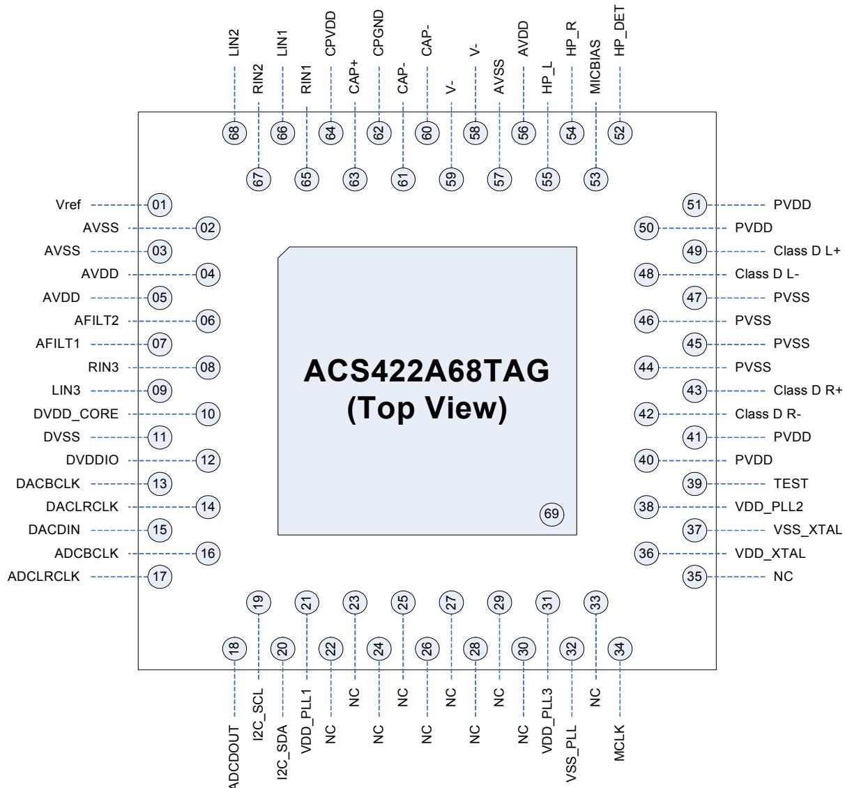
Figure 34. ACS422x68TAG Pinout
