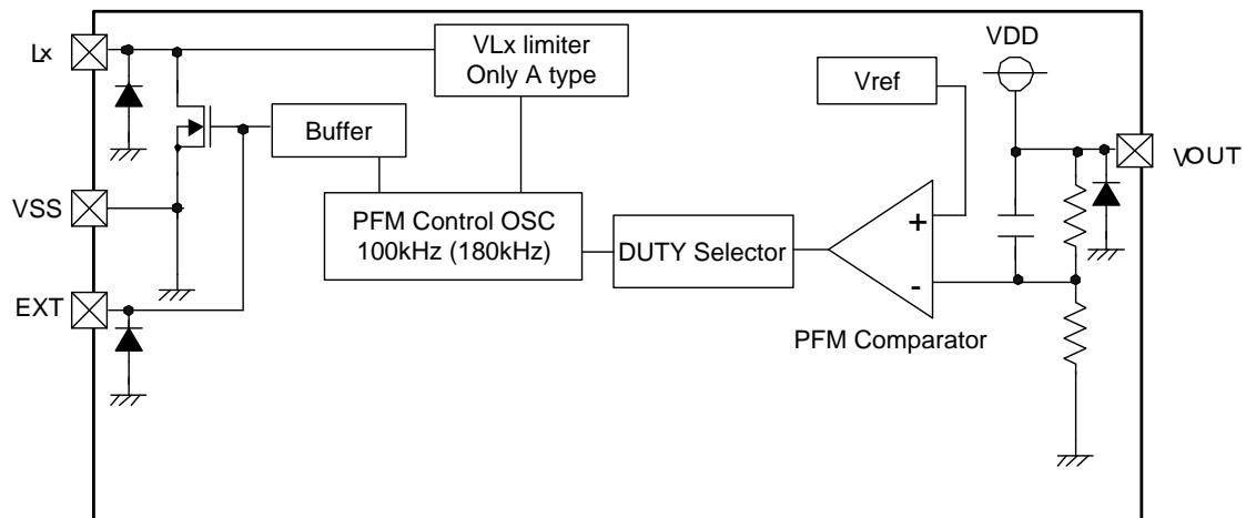
Note: The XC9110 series, Tr. Built-in type, uses the Lx pin and the XC9111 series, external Tr. Type, uses the EXT pin.
