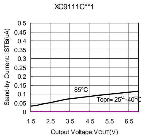
(7) No Load Input Current vs. Output Voltage
