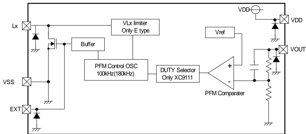
Note: The XC9110 series, Tr. Built-in type, uses the Lx pin and the XC9111 series, external Tr. Type, uses the EXT pin.
