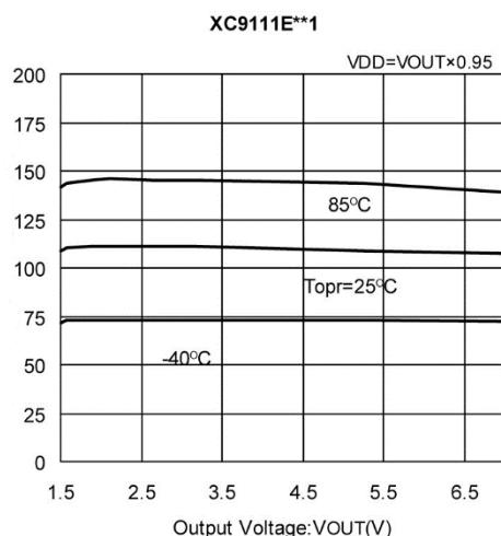
(13) Maximum Oscillation Frequency 2 vs. Output Voltage
