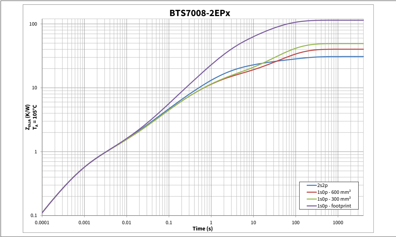
Figure 9 Typical Thermal Impedance. PCB setup according Chapter 4.4.1
