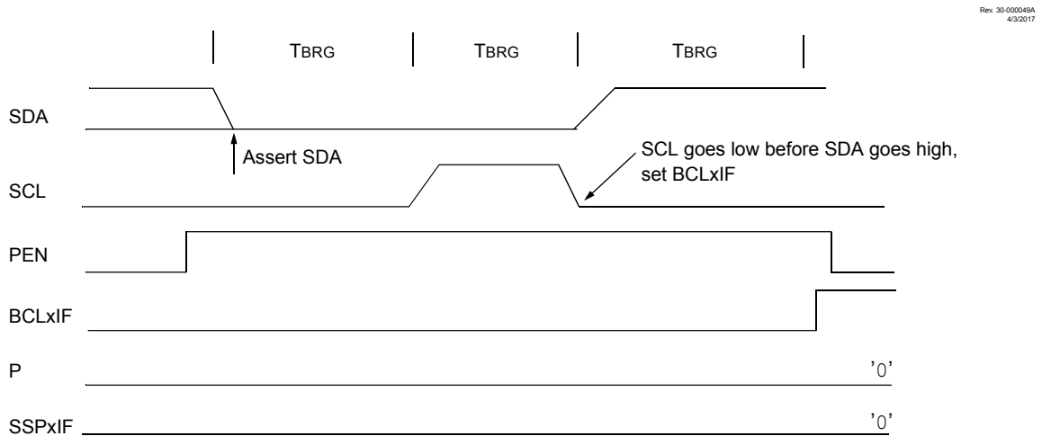
Figure 26-39. Bus Collision During a Stop Condition (Case 2)
