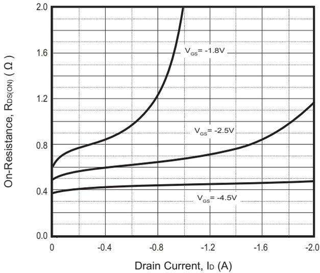
Fig.4 -  $R_{DS(ON)}$  —  $V_{GS}$
