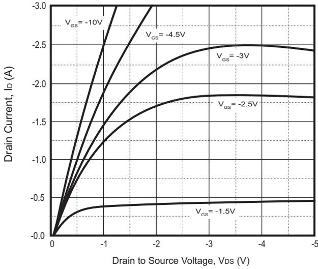
Fig.2 - Transfer Characteristics
