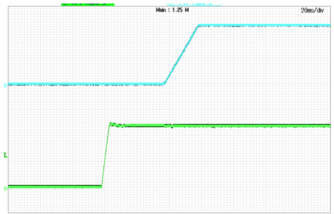
Figure 7: Turn-on transient at full rated load current (20 ms/div). Top Trace: Vout; 5V/div; Bottom Trace: input voltage: 30V/div.
