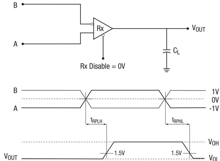
Figure 12: RS-485/RS-422 Receiver Propagation Delay
