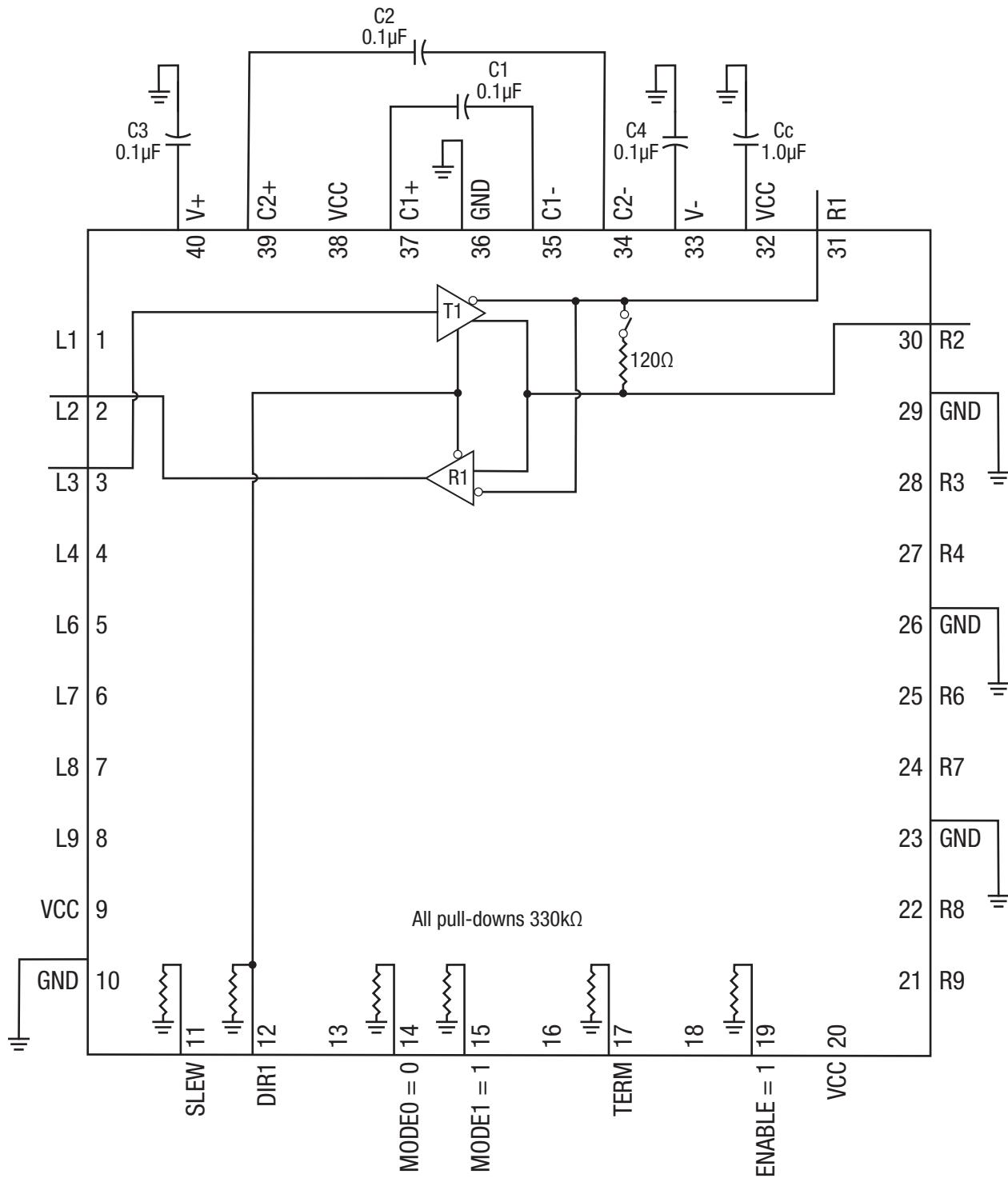
Figure 4: Functional Block Diagram - Mode 10, RS-485 Half Duplex
