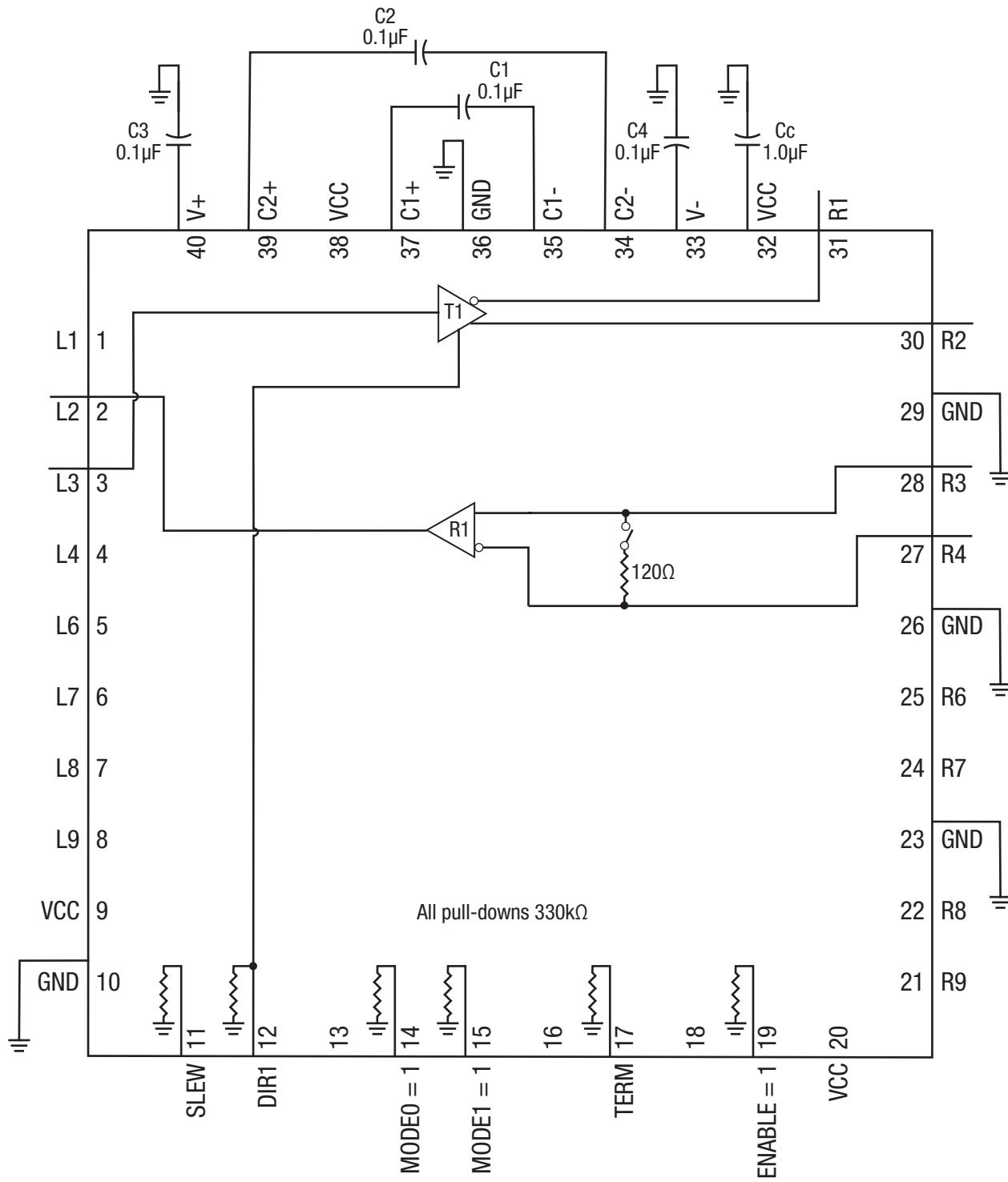
Figure 5: Functional Block Diagram - Mode 11, RS-485/RS-422 Full Duplex
