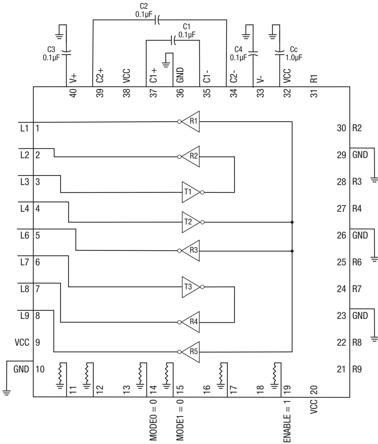
Figure 2: Functional Block Diagram - Mode 00, Loopback
