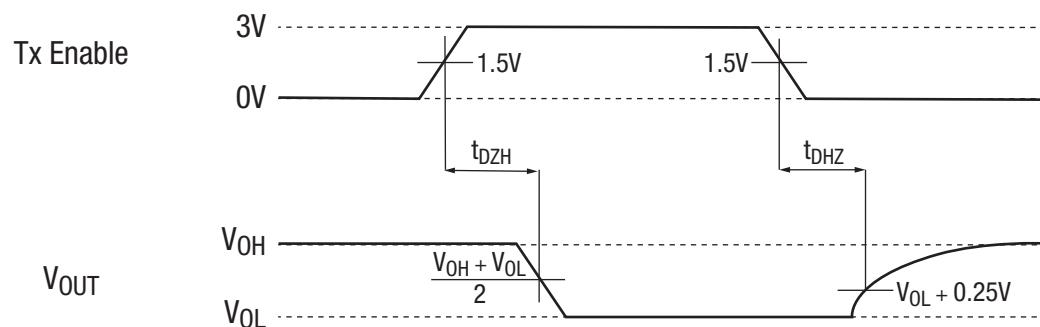
Figure 15: RS-485/RS-422 Driver Output Enable/Disable Times
