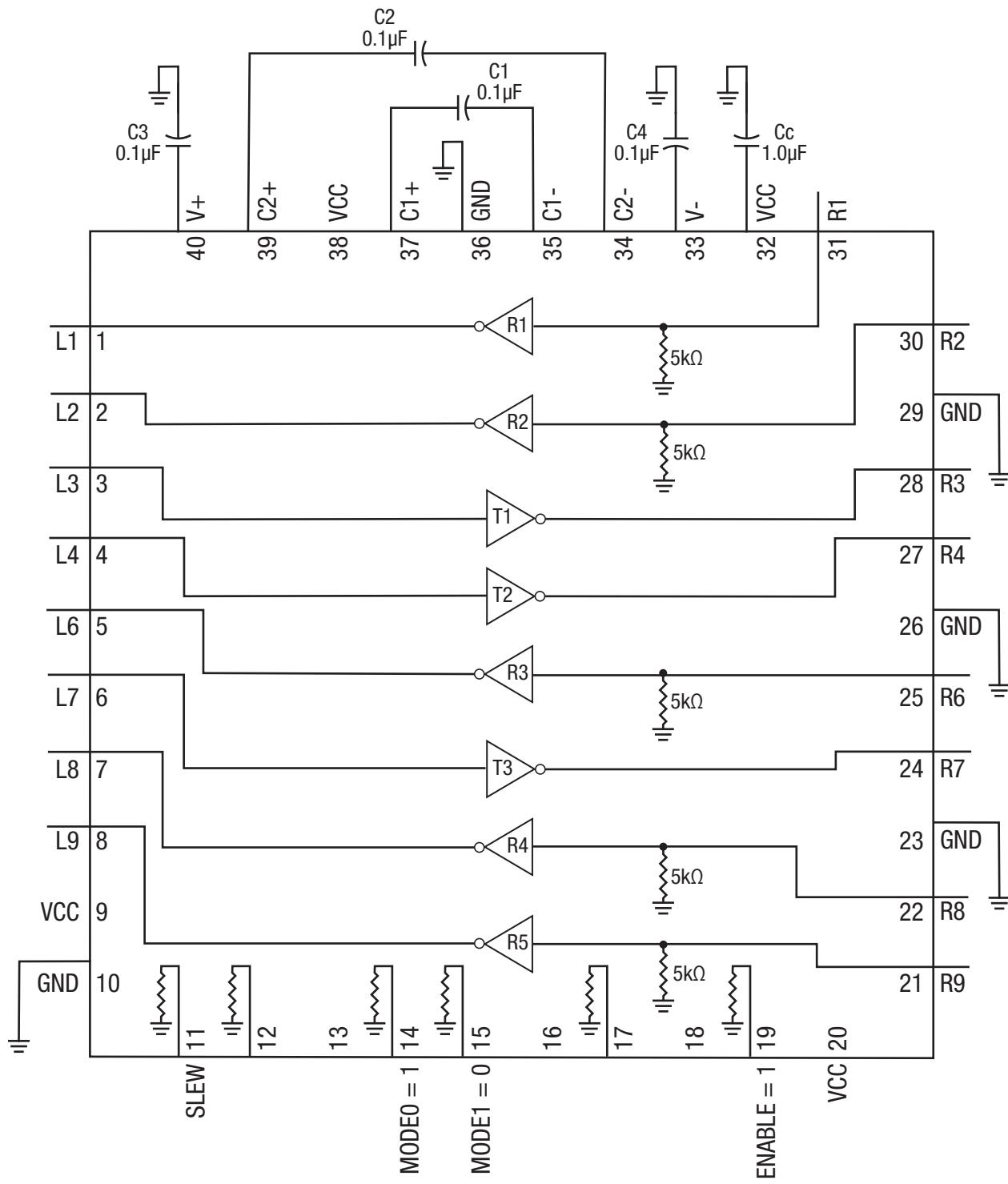
Figure 3: Functional Block Diagram - Mode 01, RS-232
