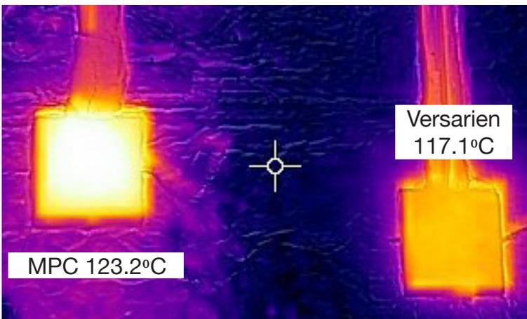
Comparative heatmap of a 40x40x2.5 microporous ceramic and VersarienCu™ heat sink at 5W. The Versarien heat sink is 6.1 $^{\circ}\text{C}/\text{W}$  cooler.
