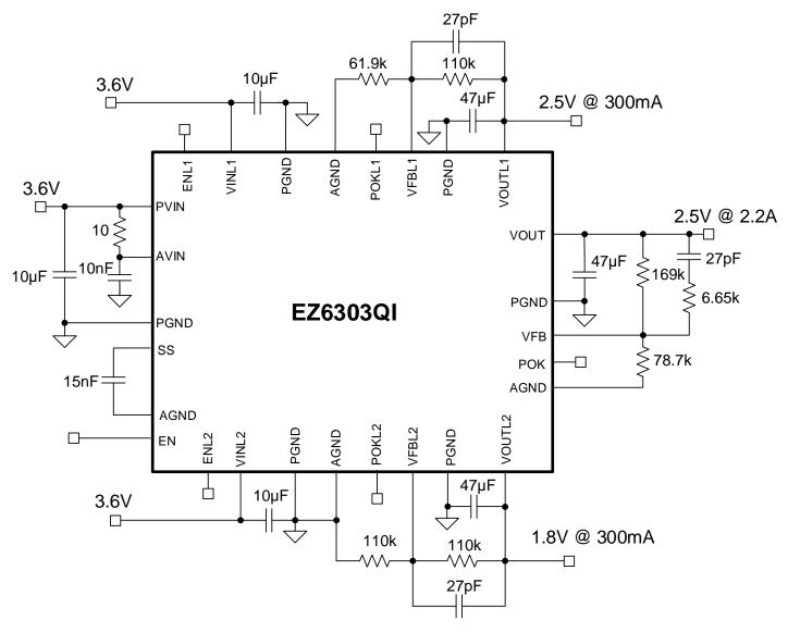
Figure 8: Application Schematic for V<sub>OUT</sub> = 3.3V, V<sub>OUTL1</sub>=2.5V, V<sub>OUTL2</sub> = 1.8V
