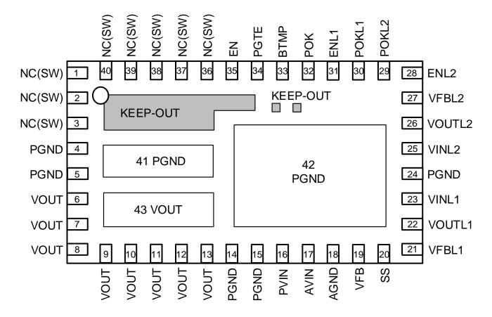
Figure 3: Pin Diagram (Top View)
