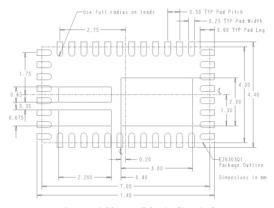
Figure 11: Solder stencil drawing (Top View)
