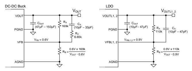
Figure 6: Output Voltage Setting (Buck left, LDO right)
