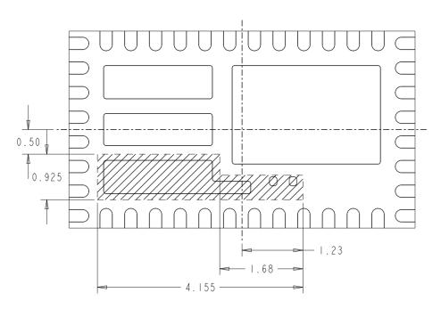
Figure 10: Lead-Frame exposed metal (Bottom View)
