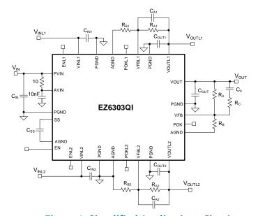
**Figure 1: Simplified Applications Circuit**
