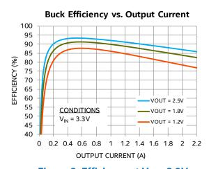
Figure 2: Efficiency at V<sub>IN</sub> = 3.3V
