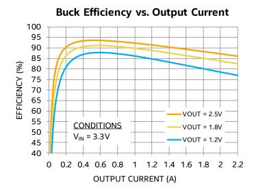
**Figure 7: Efficiency vs. Output Current**
