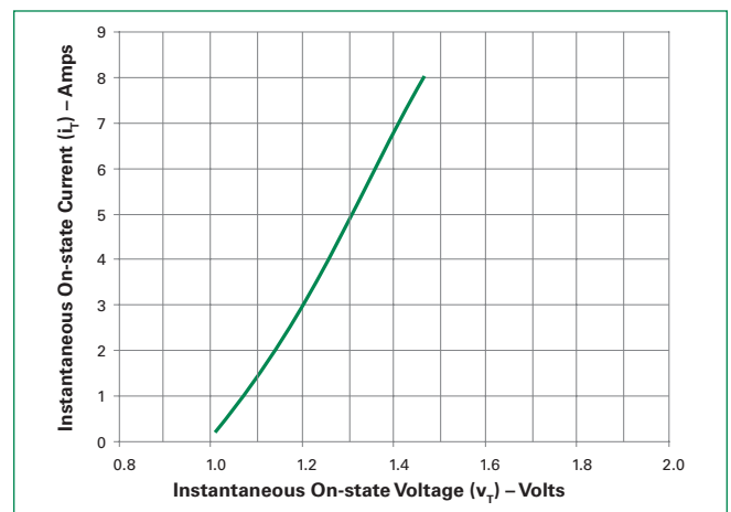
Figure 2: On-state Current vs. On-state Voltage (Typical)
