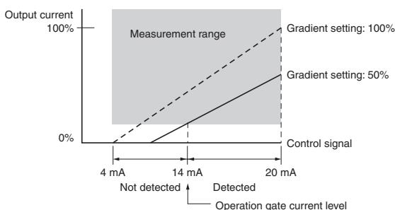
**Note:** Set the heater burnout alarm value based on the current at the heater's rated input.
