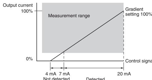
When the power regulator's gradient settings are changed, the operation gate current level is set so that the output current is within the measurement range. (In the following diagram, 14 mA is set.)
