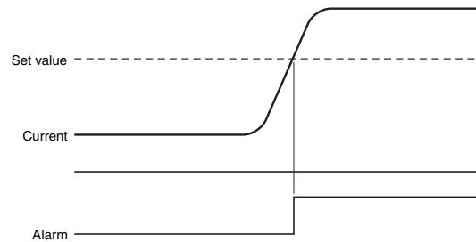
Transistor output models: ALM indicator lit, ALM transistor output
