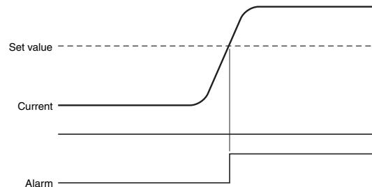
Transistor output models: ALM indicator lit, ALM transistor output
