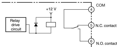
**Note:** For contact outputs, the same outputs are used for SSR error and for heater burnouts and heater layer short circuit alarm outputs.
