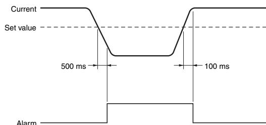
Transistor output models: ALM indicator lit, ALM transistor output
