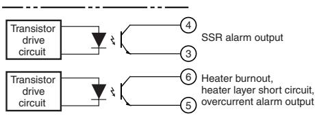
The transistor output of the K8AC-H2□□N uses a photocoupler for isolation with the internal circuits, and so either an NPN open-collector output or a PNP equivalent output can be used.
