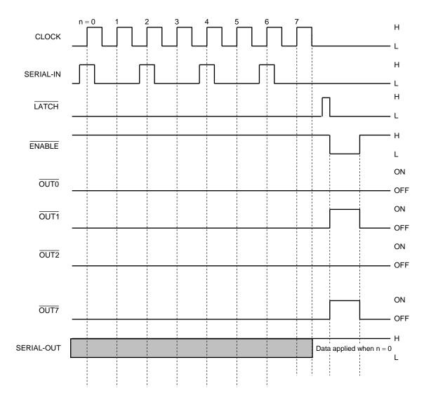
Note 1: Latches are level-sensitive, not edge-triggered.
