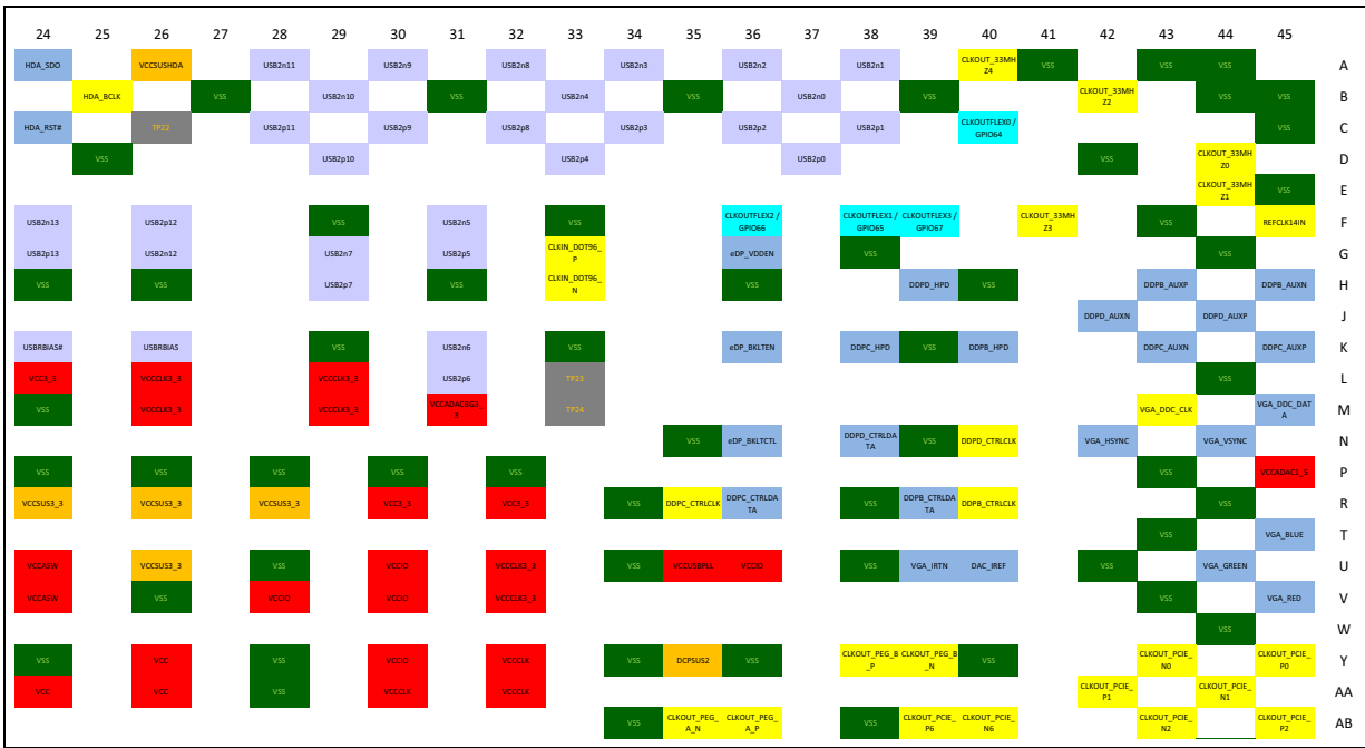
Figure 6-8. Mobile PCH Ballout (Top View - Lower Right)
