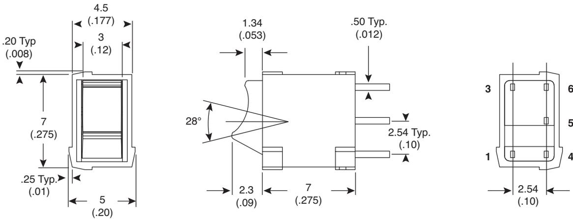
On single pole models positions 1 & 3 are support pins
