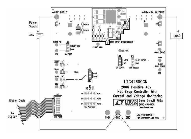
Figure 4. Proper Measurement Equipment Setup
