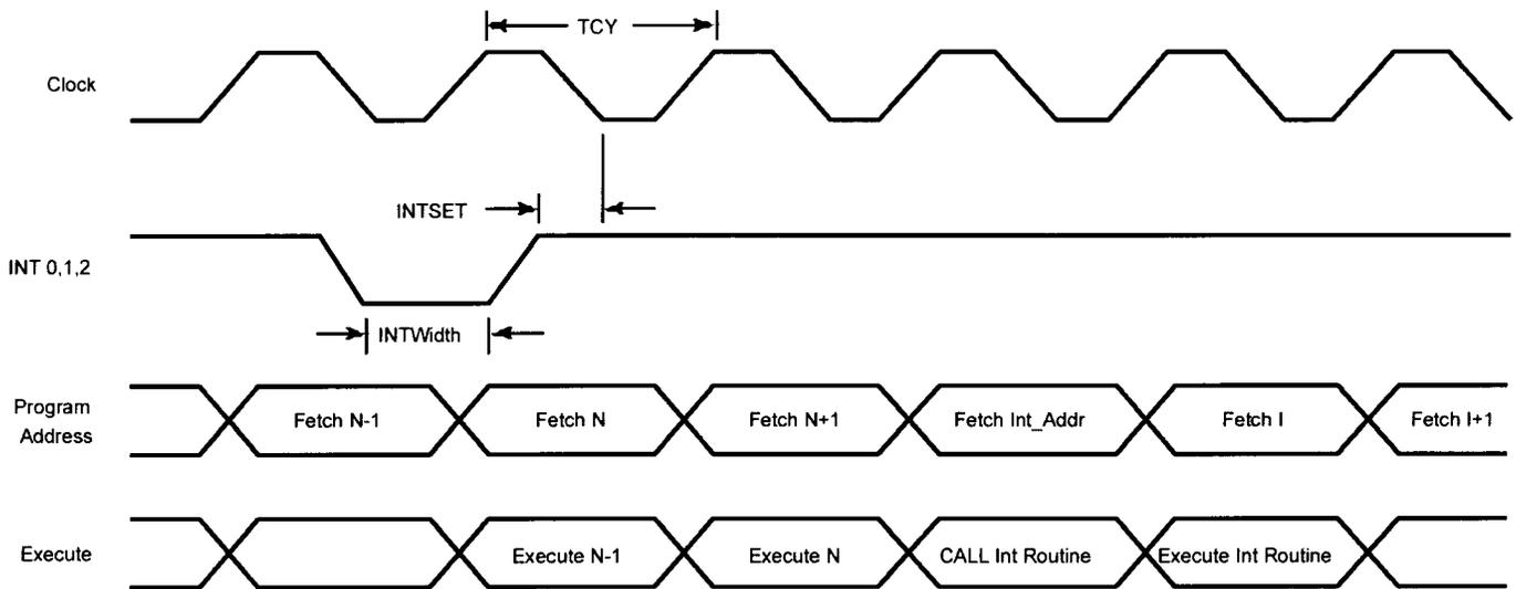
Figure 11. Interrupt Timing
